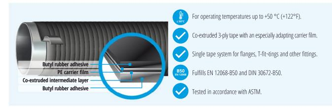
**BUTYLEN-S10** is a cold applied single tape system for corrosion prevention of metal pipes, pipelines and fittings. It is **especially suitable for uneven substrates** and **complicated geometries**.
