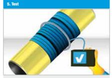
After applying the **BUTYLEN Tape** a high-voltage test can be performed according to relevant standards. We recommend the use of spiral or rubber electrodes.
