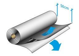
3. Now lift away the peeled separating film and press the exposed bitumen layer onto the surface. Then push the roll back so that the separating film can be removed.
