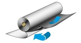
4. Applying slight tension, push the roll in the laying direction while pulling off the separating film. After laying, push the strip down onto the surface using a brush or a small roller.
