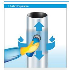
Prepare the surface carefully. Remove all rust, loose particles and loose residues of old coatings from the surface of the pile. Remove any organic substances from the surface. After cleaning the surface, proceed immediately with the coating to avoid the development of rust and organic growth. We recommend, whenever possible, to use sand or water blasting to gain best results.
