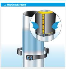
Optional: In case of coating a section of the pillar with a distance to the sea ground, a Smart® Band may be used below the first Jacket as a mechanical support. Use three Smart® Band stripes and three standard Smart® Band Buckles to form a ring as indicated in the picture. Fasten the Smart® Band with the SM-FT 2000 or SM-FT 1000 mounting tool.
