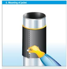
When the MarineProtect®-2000FD Jacket is fastened with all screws, an additional jacket can be mounted above the first one. Position the upper jacket with an min. overlapp of approx. 30 mm.
