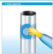
■ Apply MarineProtect®-Primer on the cleaned surface by hand, roller or using a spreading tool. Make sure that the  $complete \ surface \ is \ coated \ with \ \textbf{MarineProtect} \textbf{\$-Primer.}$ The consumption of **MarineProtect®-Primer** is about
