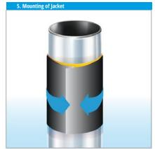
■ For mechanical protection apply MarineProtect®-100 Jacket. If the coating area of the pile is higher than 1.9 m several jackets may be used. Start mounting the lower jacket. We recommend to install the shorter jacket first. Prepare the Smart® Band sections (circumference + min. 5 cm) per Jacket. The length of the jacket allows a sufficient overlap. The overlap of the jacket should not face the breaking waves.
