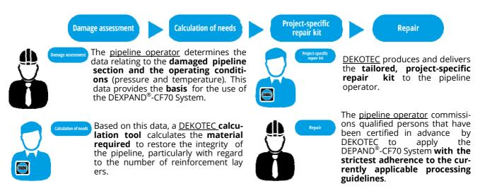
The system has been specifically developed for the repair of pipeline systems. It is not suitable for the repair of leaks. Please refer to the application recommendation available separately.
